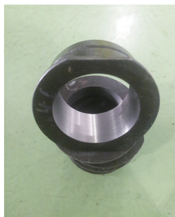
图6 加工后的试刀衬套 Fig.6 Trial bushing after processing
